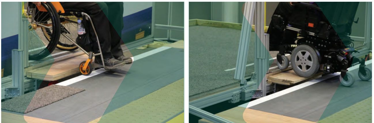
Figure 4: HS2 Ltd level access boarding trials.
