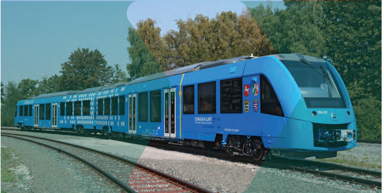
Figure 8: Alstom's zero-emission Coradia iLint train.
