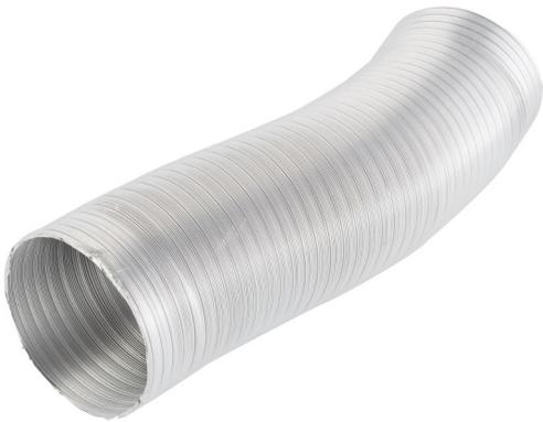
**MATERIAL:** An aluminium foil hose with no reinforcement. Manufactured from an aluminium strip spirally wound to produce a double overlapped joint, which is crimp-locked by a unique patented process. The extra deep corrugation of the aluminium duct brings a new flexibility to the metal tube. The duct is self supporting and will not sag when compared to fabric flexis.
