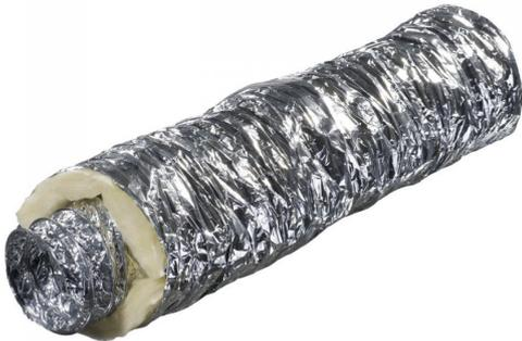
**MATERIAL:** Aluminium hose with thermal insulation 25mm glass wool insulation. Developed to minimise heat gain or loss resulting from temperature differential between the airflow and the surrounding ambient air. Produced from multi-layer aluminium and metallized polyester, strengthened with high tension hard steel wire, surrounded with glass wool insulation and an aluminium vapour barrier. Manufactured to BS476 Part 6&7 Class O
