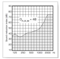
The diagram shows the sound reduction performance with the vents fully opened. Calculations are based on area of  $10m^2$
