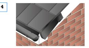
Slide the first verge unit over the tile at the eves and into the starter kit, fitting it under the headlap to ensure the unit is firmly held in place. Screw fix the unit through the top grid into the batten.
