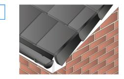
Continue the process up along the barge board unit at the ridge. If required insert the blanking plate over the final nail grid to prevent water ingress. Finally insert the ridge cap once the verge is completed.
