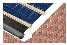
Install the tiling batten with a 30mm overhang over the brick or barge board. Remove existing mortar bedding in refurbishment projects and install new tiling batten to the underside of the existing tiling batten.
