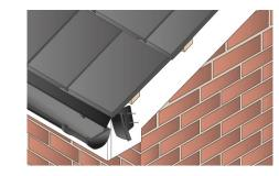
Snap the starter kit off the blanking plate. Starting at the bottom edge, insert the starter piece into the front end of the verge unit. Mark starter position on barge. Remove unit and mechanically fix into position through holes provided.
