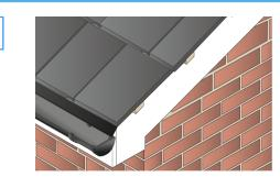
Lay tiles flush with battens. Remove existing mortar bedding in refurbishment projects.
