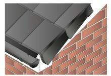
Slide the next verge unit into the upper edge of the first unit, press firmly to the tile while fitting it under the head laps to ensure the unit is firmly held in place and then nail the unit through the top grid into the batten.
