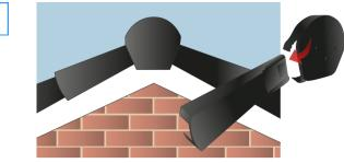
Ensure the flexible flaps on the ridge cap contour around the outside of the verge unit. Fix the ridge cap to the battens.
