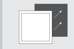
Offer the panel to the prepared cut out hole, pressing firmly into place to ensure the panel fits the cut out ope.
