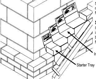
**5.** When the wall and trays are complete, the lead flashing should be dressed down into position. It will be necessary to dress additional soaker lead or similar from the roof covering up under the cavity tray lead flashing for extra protection.
