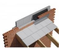
2. Ensure weep vents are fitted at approximately 900mm along the cavity tray in the mortar joint to discharge excess water and to comply with Building regulations. Keep the cavity trays and weep holes clean and free from mortar droppings.
