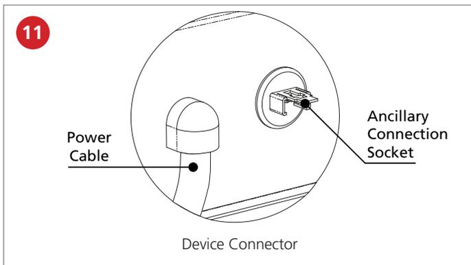
If an ancillary is to be used, the cable can be connected to the backside of the MVHR unit via the ancillary connection socket (Figure 11). Refer to the relevant ancillary installation manual for more details.
