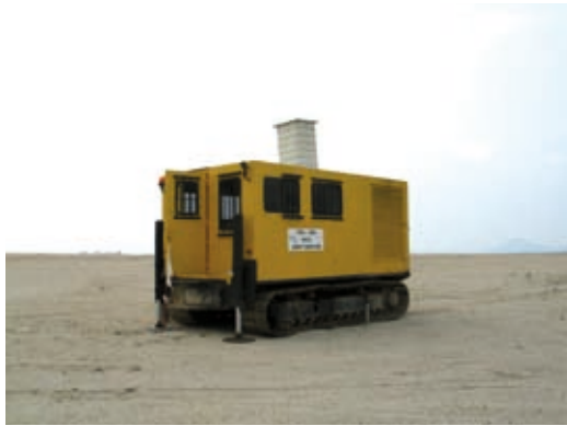
Machine to measure the softness of the new ground
