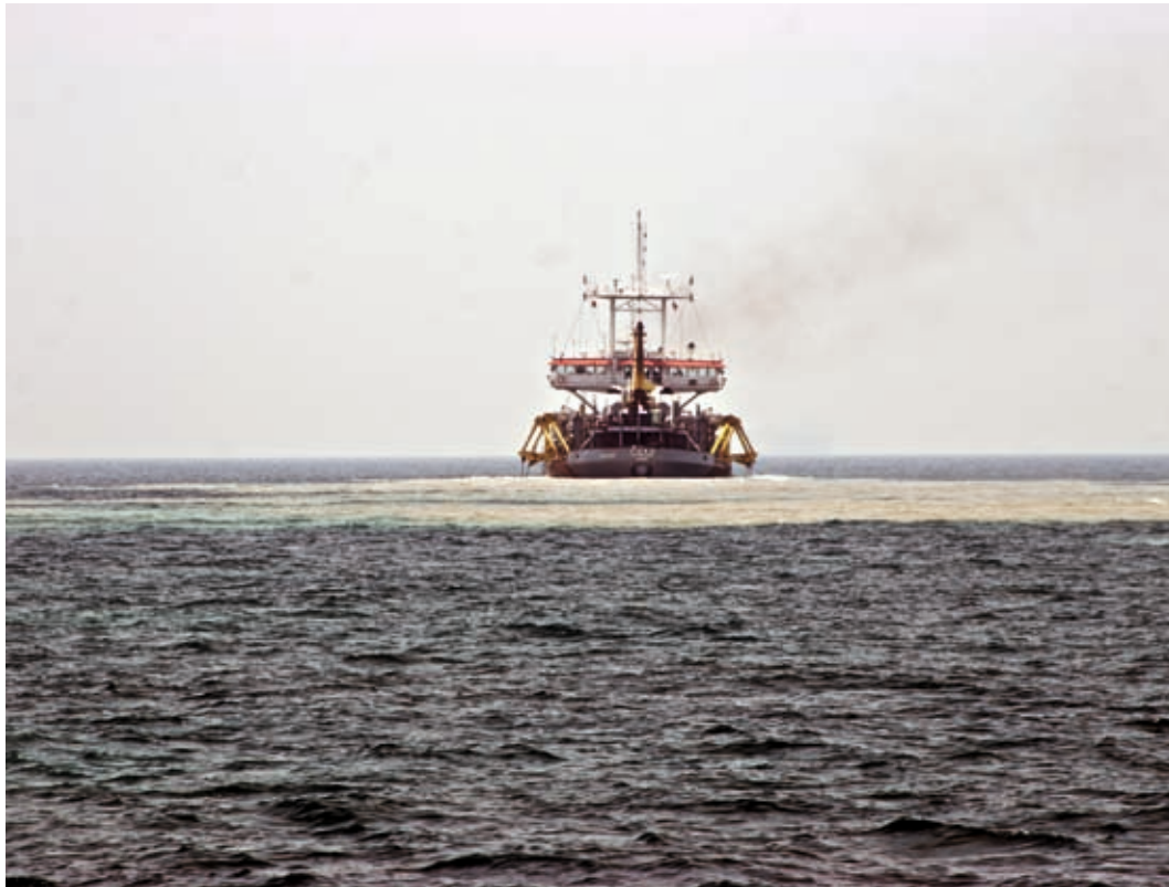
Hyundai dredging ship designed to suck sand from the seabed
