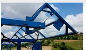
The most important innovation in the design of the bale trailer, unlike in previous models, are hydraulically lifted side walls to protect the transported cargo. The large loading surface of the trailer and its optimal load capacity makes it possible to transport a wide range of different materials and to use the trailer not only in agriculture
