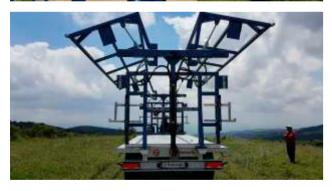
Hydraulic side walls can flex up to 3 meters nad can up to 90°. 4 mm platform and strong design created for hard conditions.
