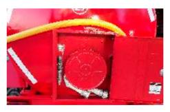
Fire tanks are almost same with water tanks except some equipment for fire fighting. We apply pressure fire noozle, 20 meters pressure cloth hose, fire box and 360° turning water monitor. Pump is standart 2" centrifugal pump and Works with PTO shaft or motopomp.
