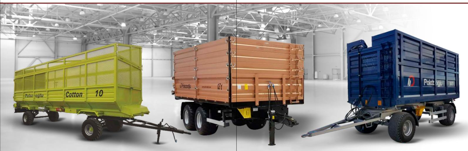
Long platfrom and high sideboards created for cotton transport solutions. Sideboards made by perforated sheet to make trailer lighter. This trailer has 2 option for unloading.
