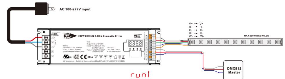
**Note:** Please make sure that the stripped wires are fully inserted into the terminal blocks and screws are tightened!
